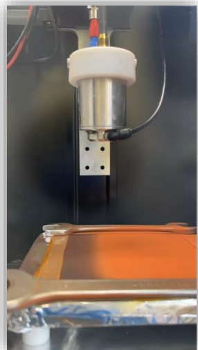
GDE preparation by spray coating
